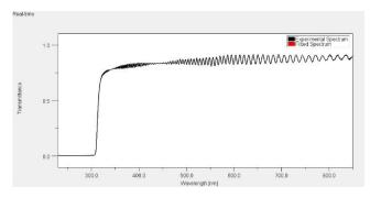
**Figure 2.** Transmittance spectrum of a cling film at the 220-850nm region.
